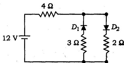
The circuit given above has two oppositely connected ideal diodes in parallel. What is the current flowing in the circuit?
