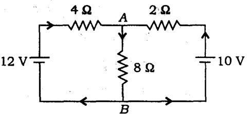
What is the value of current passing through the branch AB in the electric circuit given above?
